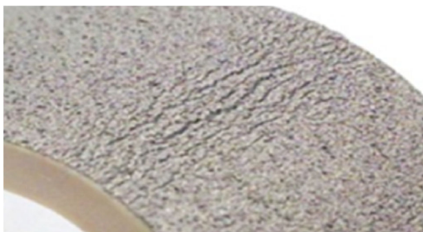
Figure 3. EN ISO 7438 bending tests of six plasma-spray-coated implant surfaces clearly show cracks in the coating layer. A further consequence may be delamination/abrasion. In-house research.
